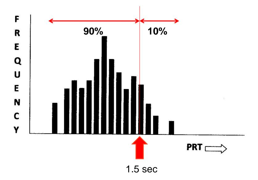
2.5 seconds "... large enough to include the time taken by nearly all (90% of all) drivers under most highway conditions."
