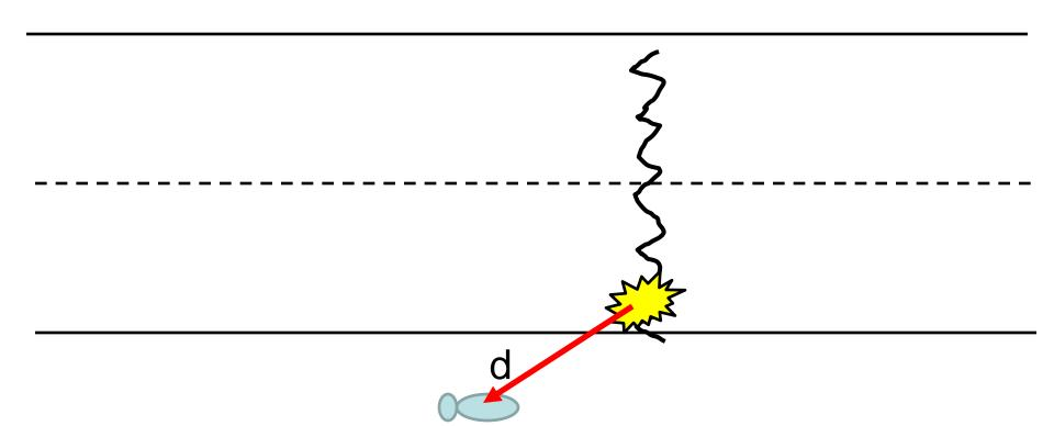
$$V_{min} = \sqrt{\frac{2 \text{ f g d}}{1 + f^2}} \qquad d \approx 15 \text{ ft}$$
